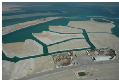
Apart from this 6,5 Mio m<sup>3</sup> was dredged by means of a CSD and delivered to the reclamation area via a floating pipeline, sinker line and shoreline. In the borrow areas layers of hard rock occurred next to pockets of soft silt, the latter being unacceptable as such for use as reclamation material. As selective dredging was not acceptable due to its major impact on the dredger's efficiency the Contractor opted to treat these fines within the reclamation area. Via the technique of "finger
